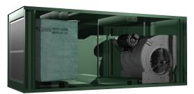
The CamCleaner air cleaner is also available with a filters specific to the removal of mists (including oil). Filters include a Camfil metal mesh mist removal filter and a MERV 13 Hi-Flo® ES bag filter. The unit includes a 1" IPS drain connection for mist collection for reclaim or disposal.
